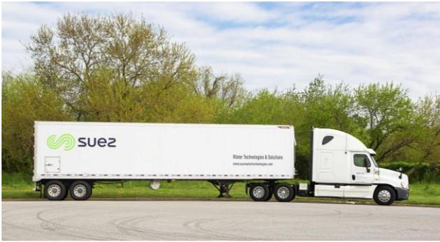
**Figure 1: SUEZ’s MobileFlow demineralization trailers.**
