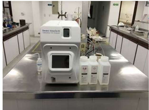
Figure 1. Sievers* InnovOx Laboratory TOC Analyzer used for Leak Detection
