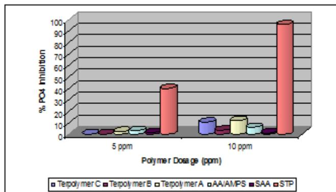
**Figure 1: Calcium phosphate inhibition at 400 ppm calcium hardness, pH 8.2, 10 ppm PO<sub>4</sub>, 160°F (70°C)**
