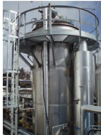
The poseidon VOWS is based on the well-proven poseidon Saturn DAF/DNF design.
