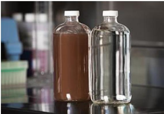
**Figure 3: Untreated wastewater from CRC (left) and SUEZ-treated wastewater (right)**
