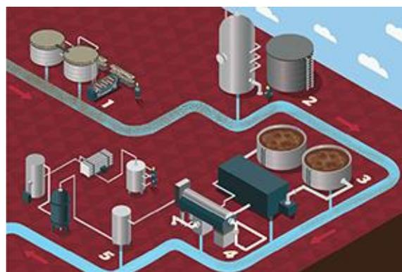
**Figure 1: The CRC Wastewater Improvement Project features a five-stage wastewater treatment solution that enables the recycling and reuse of 2 million gallons of wastewater a day.**
