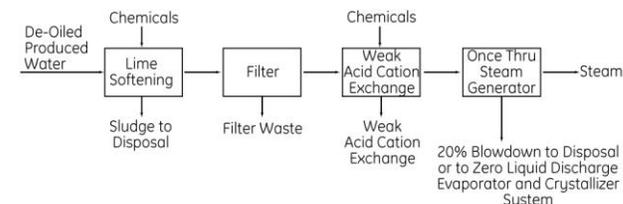
**Figure 1: Traditional Produced Water Treatment System**
