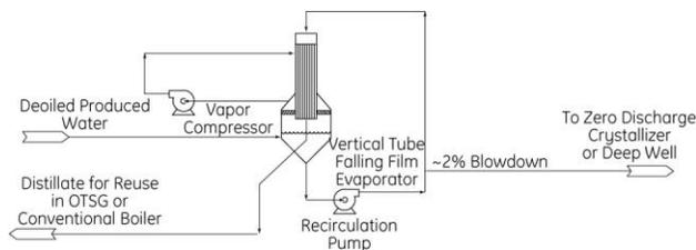
**Figure 3: Simplified Vapor Compression Falling Film Evaporator System**
