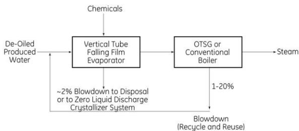
**Figure 2: Vertical Tube Falling Film Vapor Compressor Evaporator System**
