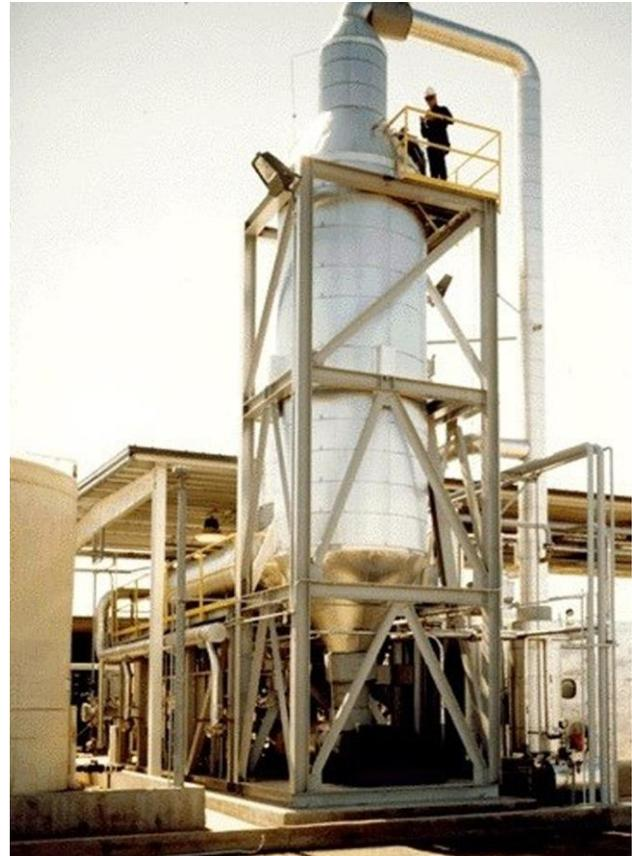
**Figure 6: Typical ZLD RCC Crystallizer System**
