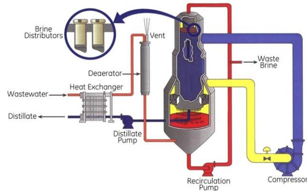
**Figure 4: Vertical Tube Falling Film Vapor Compression Evaporator Schematic**
