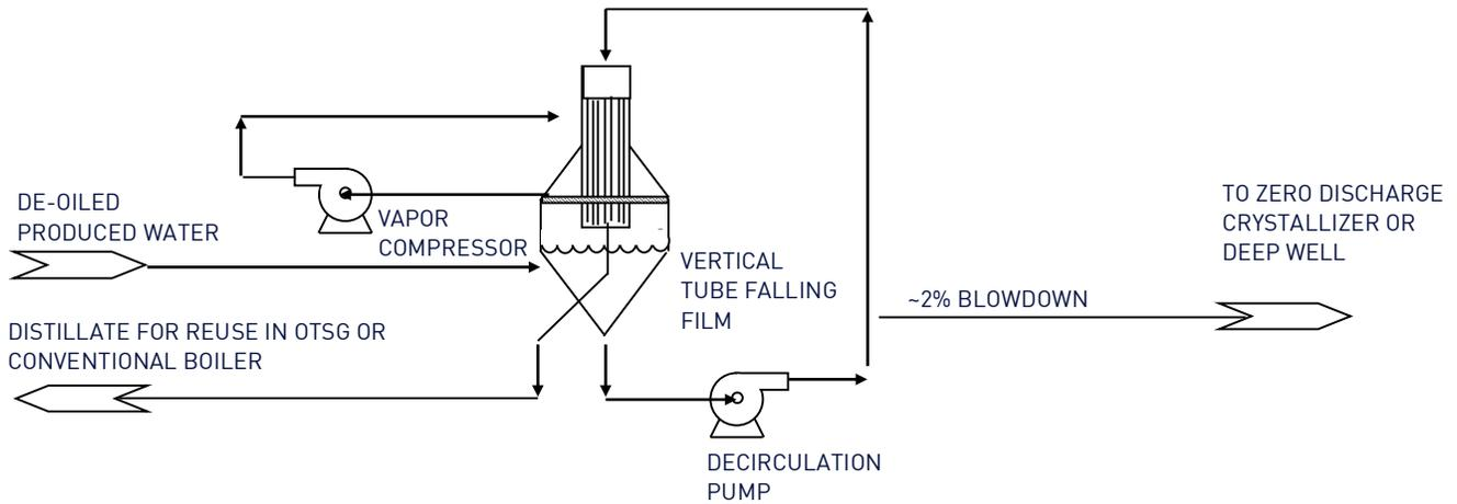
**Figure 3: Simplified Vapour Compression Falling Film Evaporator System**
