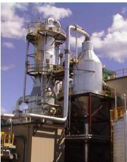
Figure 6: Typical SAGD Zero Liquid Discharge Evaporator and Crystallizer System
