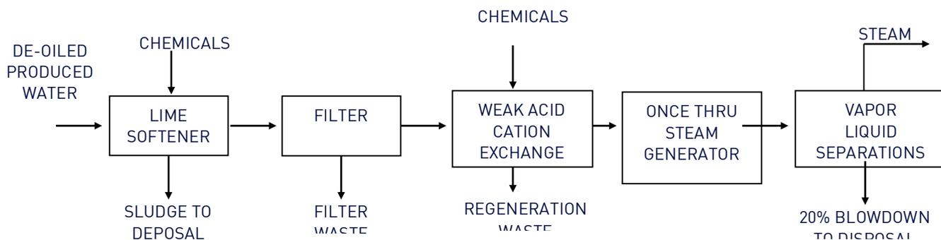
Figure 1: Traditional Produced Water Treatment and Steam Generation System
