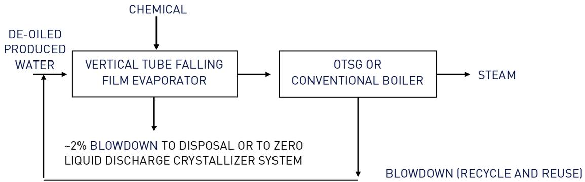
**Figure 2: Evaporative SAGD Produced Water Treatment and Steam Generation System**
