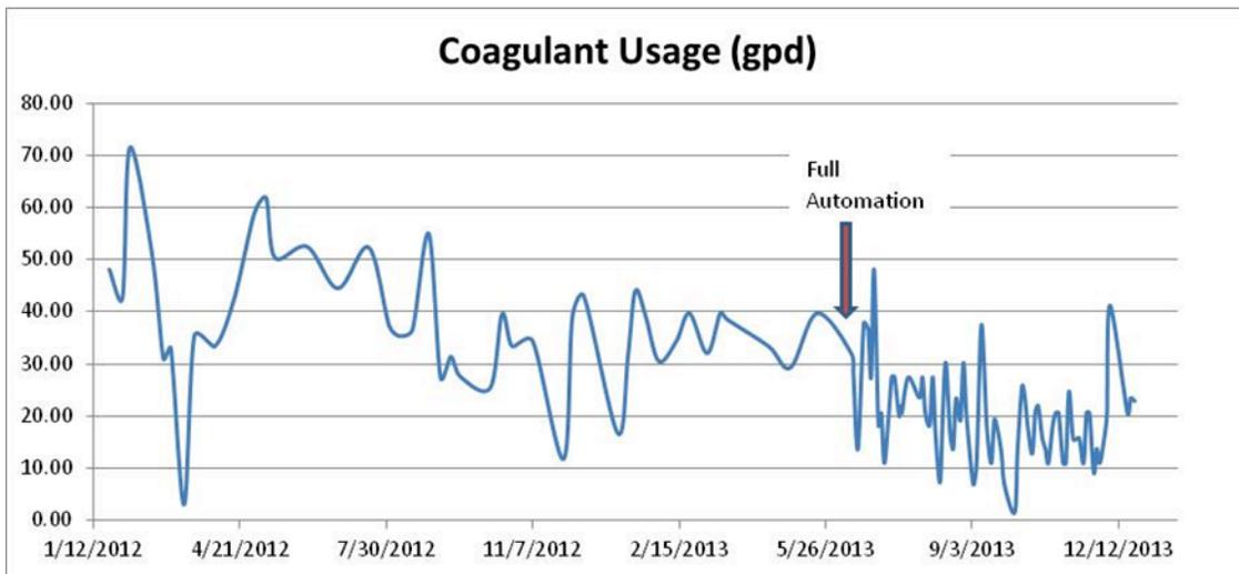
**Figure 3: Chemical usage before and after full automation with influent turbidity and flow**
